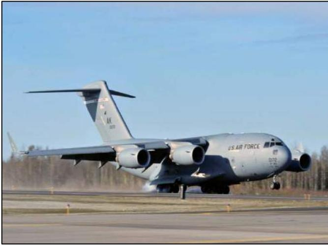
The C-17 is approximately 174 feet long and has a wingspan of 169 feet, 10 inches, and its maximum takeoff weight is 585,000 pounds. It is powered by four, fully reversible F117-PW-100 (Pratt & Whitney PW2040) engines, each producing 40,440 pounds of thrust. The C-17 can cruise at 450 knots (kts), and its range is global with in-flight refueling.
